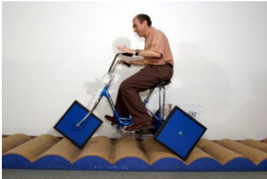
Stan Wagon rides his square-wheeled trike over a special roadway.
