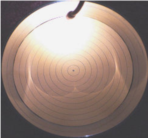
Figure 1: Caustic inside a cylinder with the light part of the way from the circumference to the center.
